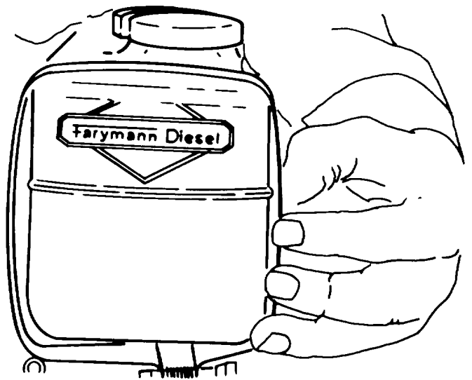
Figure A-64. Fuel Tank
